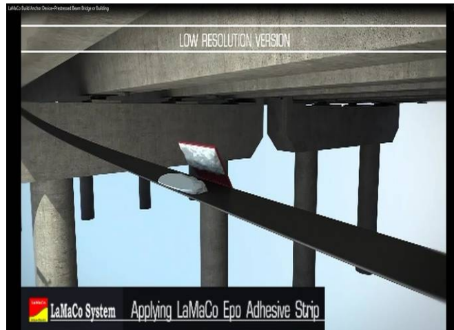
14] Laying the LaMaCo-Epo Adhesive Strip
