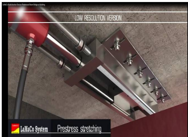
15] Jack Pump for Prestress Stretching
